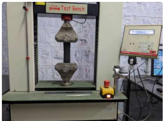
Figure 2: Tensile testing on NBR coated Nylon 66 fabric-reinforced composite
