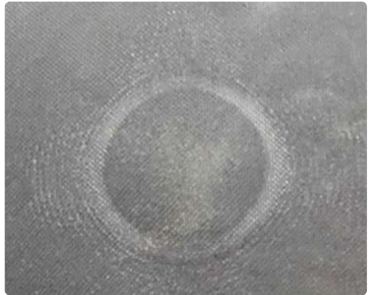
Figure 3: Hemispherical shape obtained from burst test
